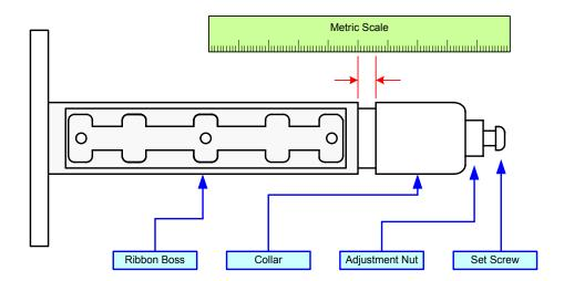
Figure 6-8, Ribbon Spindle Tensioning
